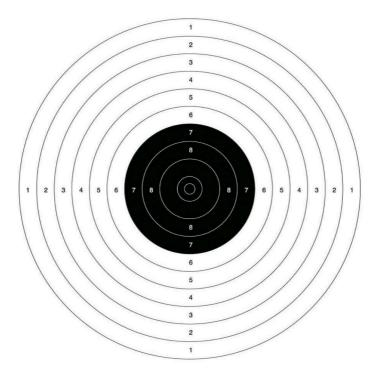
Central ten: 5.0 mm (+/- 0.1mm) Black from 7 to 10 rings = 59.5 mm Ring thickness: 0.1 mm to 0.2 mm Minimum visible size of target card 170 mm x 170 mm
